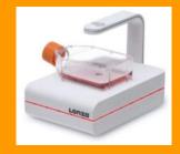
The CytoSMART system fits inside an incubator and allows for remote cloud-based imaging and monitoring of cell health, cell growth & confluence. It can be used to monitor hypoxic cell growth & cell migration. It can even alert users on a PC, smartphone or anywhere with web access when the culture reaches a desired confluence!
